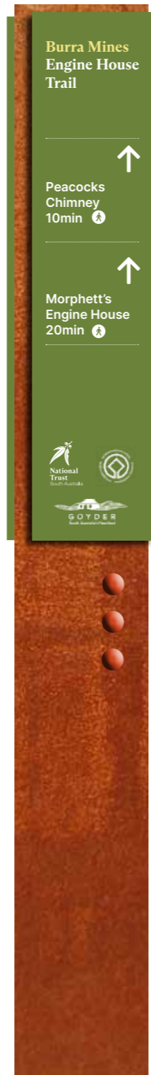
2 SIGN BODY SHS 1000X125x125mm SIGN FACE 115x490x3mm (4 SIDED)
